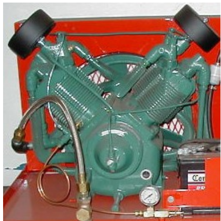
(a) V-type Two Cylinder
