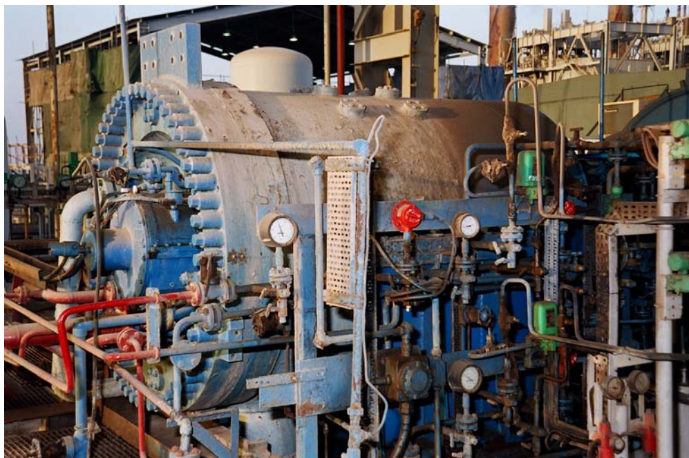
(b) Vertically-split Process Stage 4
