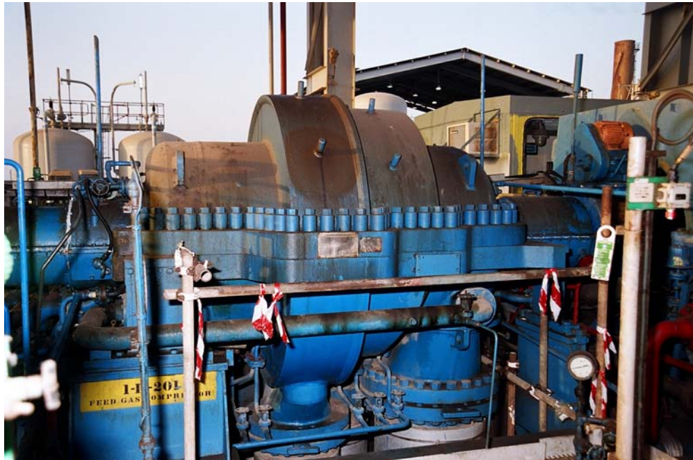
(a) Horizontally-split Process Stages 2 and 3
