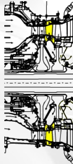
HPT Nozzle 2 cooling
