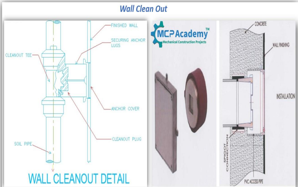
Cast Iron Wall Clean out
