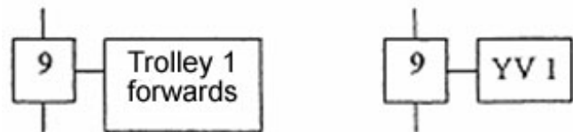
Figure 54 : Example of an action associated with a step (step No. 9 here)
