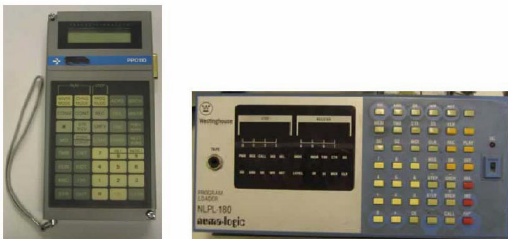
Figure 30: Examples of programming consoles
