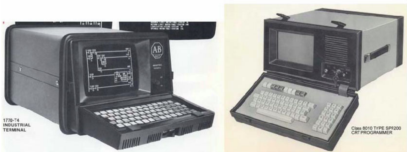
Figure 31: Examples of microcomputers dedicated to programming
