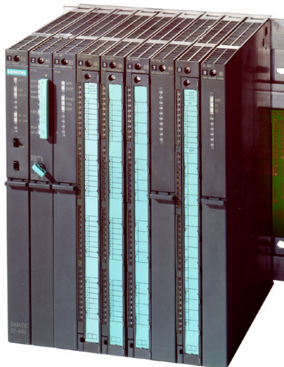
Figure 2: SIEMENS S7-400 PLC
