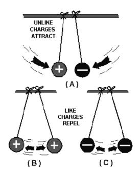
Figure 1-6.—Reaction between charged bodies.
