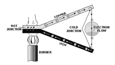
Figure 1-21.—Voltage produced by heat.
