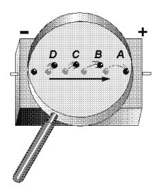
Figure 1-26.—Effect of directed drift.
