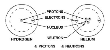
Figure 1-1.—Structures of simple atoms.
