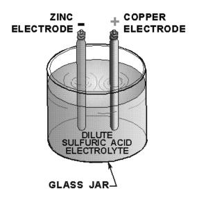
Figure 1-23.—Voltaic cell.
