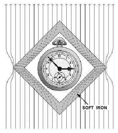
Figure 1-18.—Magnetic shield.
