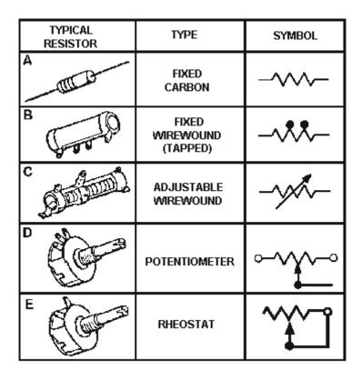
Figure 1-29.—Types of resistors.
