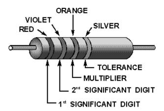
Figure 1-31.—Resistor color codes.
