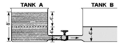
Figure 1-19.—Water analogy of electric differences of potential.
