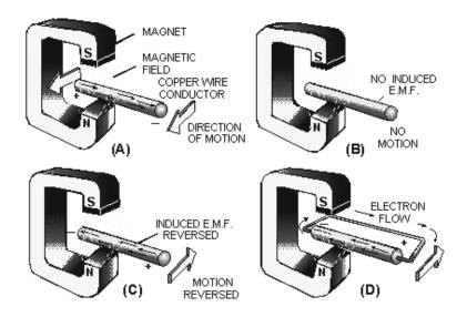
Figure 1-24.—Voltage produced by magnetism.
