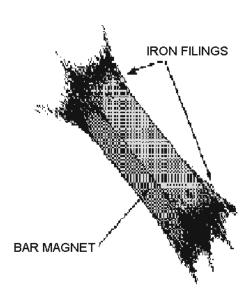
Figure 1-8.—Iron filings cling to the poles of a magnet.
