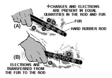
Figure 1-5.—Producing static electricity by friction.
