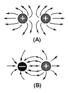
Figure 1-7.—Electrostatic lines of force.
