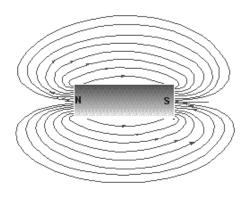
Figure 1-14.—Bar magnet showing lines of force.
