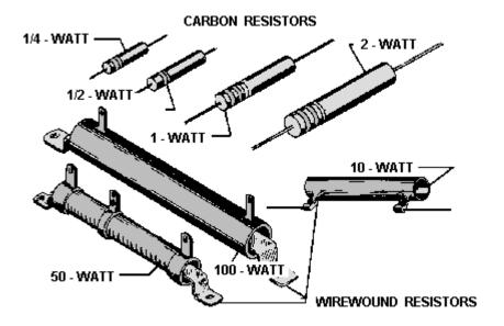
Figure 1-30.—Resistors of different wattage ratings.
