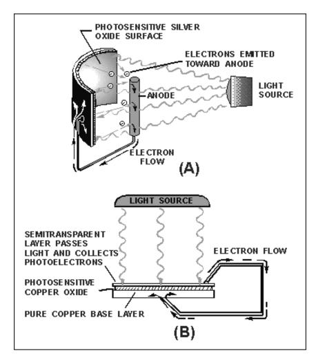
Figure 1-22.—Voltage produced by light.
