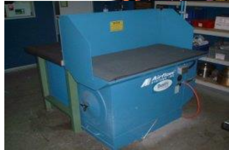
Downdraft Table For Seal Dis-assembly Work
