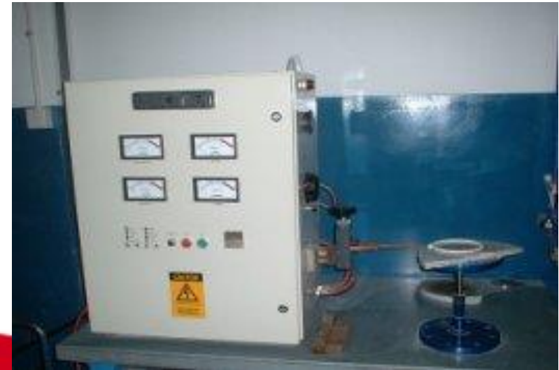
Induction Heater For Bellow Seal Face Replacement
