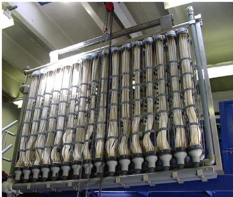
Figure 3: Membranes destined for installation at one of the MBR sites currently under construction
