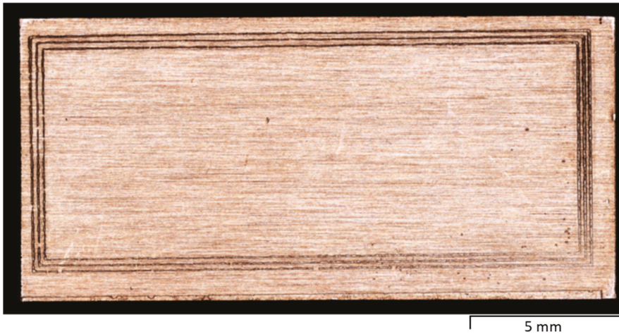
Figure 12. Oxygen-free copper substrate for thermal spreading in the package of hollowed GaN chips after micro-embossing.
