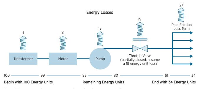
Figure 7. Energy losses in a pump system when a throttle valve controls flow
