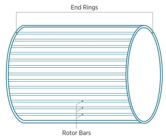
Figure 3. Squirrel-cage rotor
