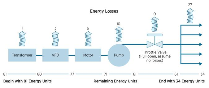
Figure 8. Energy losses in a pump system when an ASD controls flow
