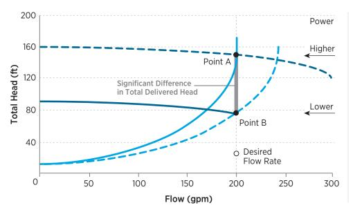
Figure 6. Effect of speed reduction on the power used by a pump
