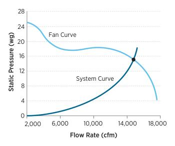
Figure 9. Typical fan and system curves
