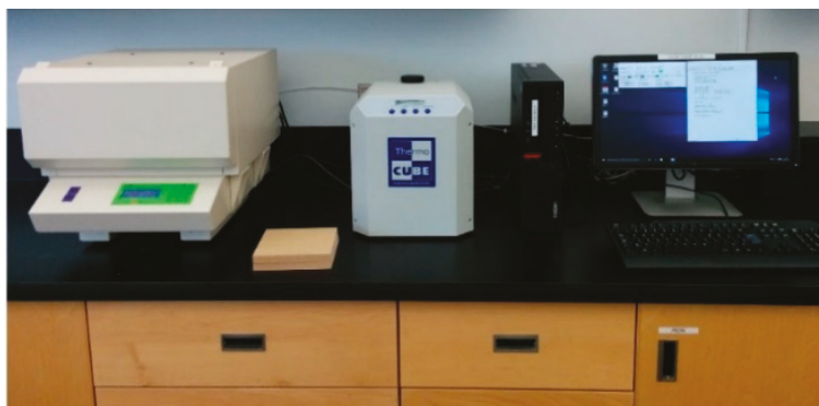
Figure 7. Equipment for thermal conductivity measurements.
