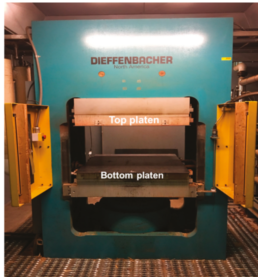
Figure 1. Steam injection hot press used for THM densification treatment.
