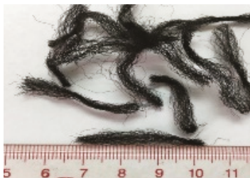
Figure 1. Waste PP fibres with 30 mm length.
