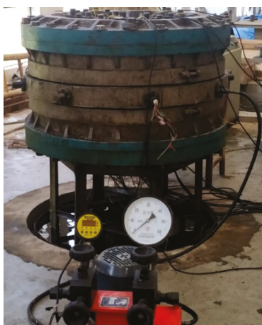
Figure 11. Shaft lining structure high-pressure loading device.
