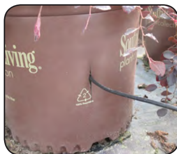
Figure 39. Moisture sensors are placed directly into the container to measure substrate moisture level
