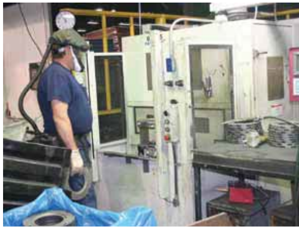
Figure 14. Machining Castings on CNC 1
