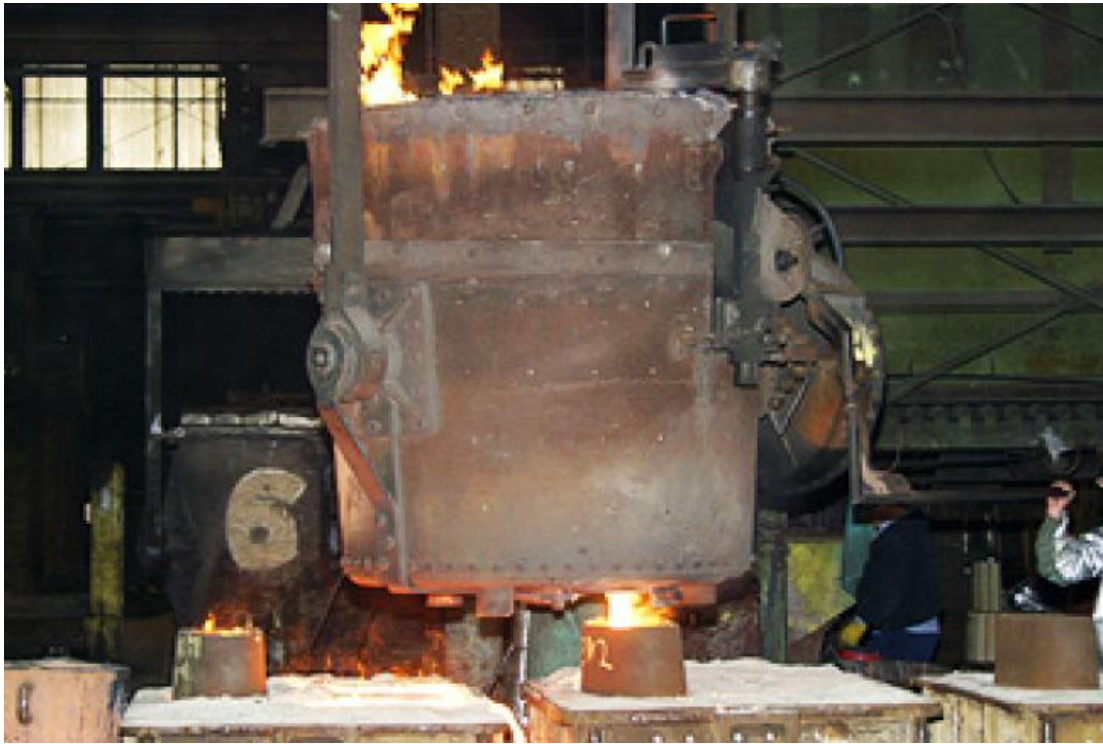
Figure 8. Ductile Iron is Poured into Molds 1
