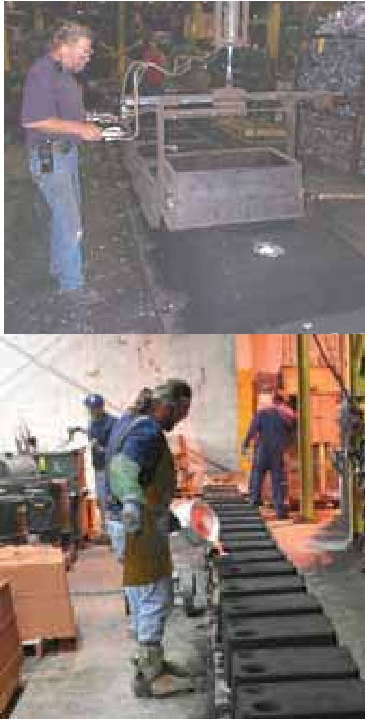
Figure 6. Sand-Clay Mold on Conveyor 1
