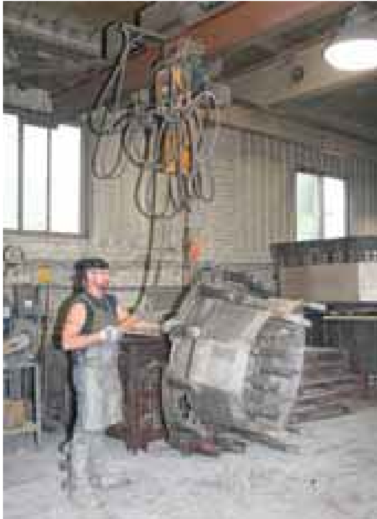
Figure 9. Large Castings Being Removed from Mold 1
