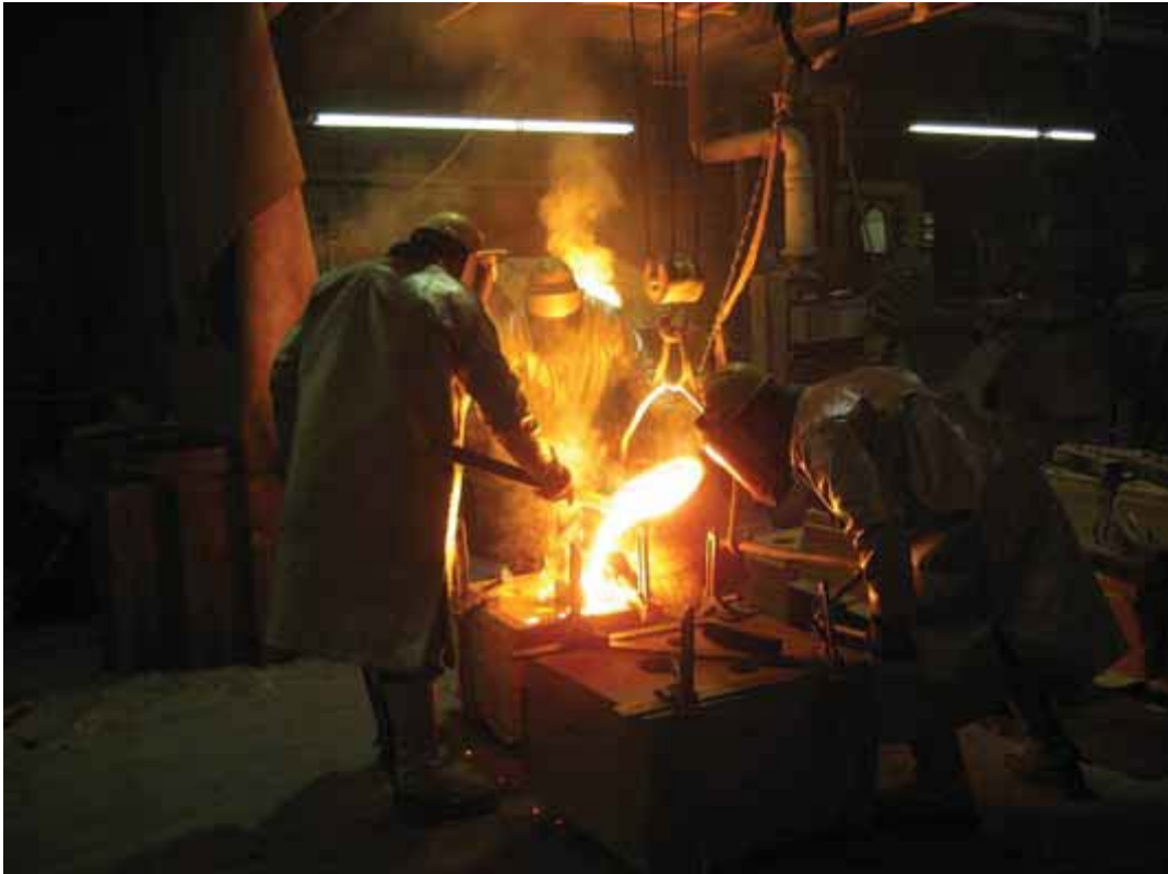
Figure 7. Metal Casting in Foundry 1
