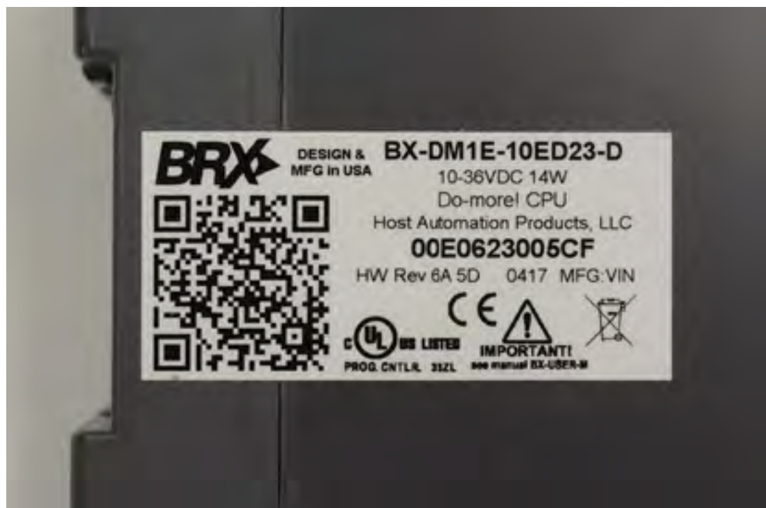
Figure 4A: Quality-built home and industrial electronic devices have marks indicating they have passed a variety of tests. The UL mark shown here indicates extensive evaluation and testing.
