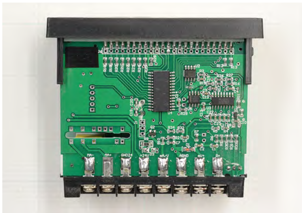
Figure 4C: The internals of an unbranded, uncertified temperature display. It carries no marks at all, so there is no assurance it was designed well, uses quality components, or was assembled properly. For example, the MA+ connection (second from left) does not appear to be soldered, and the adjacent connections are hand soldered and inconsistent.
