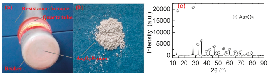
Figure 3. (a) Arsenic removal from mixed ore by roasting in resistance furnace with quartz tube under air atmosphere and 1000 °C; (b) Collected \text{As}_2\text{O}_3 powers condensed in cold beaker; (c) XRD spectra of collected \text{As}_2\text{O}_3 powers condensed in cold beaker.
