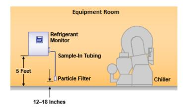
Typical Refrigerant Monitor Installation
