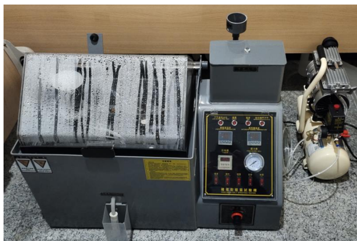
Figure 1. Salt spray tester with air compressor.
