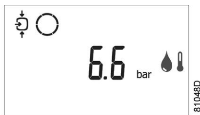
Main screen with the dewpoint temperature warning
