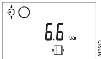
Main screen with shut-down indication, motor overload
