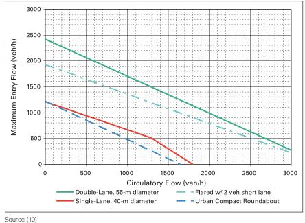
Exhibit 4-6. Capacity comparison of single-lane and double-lane roundabouts.
