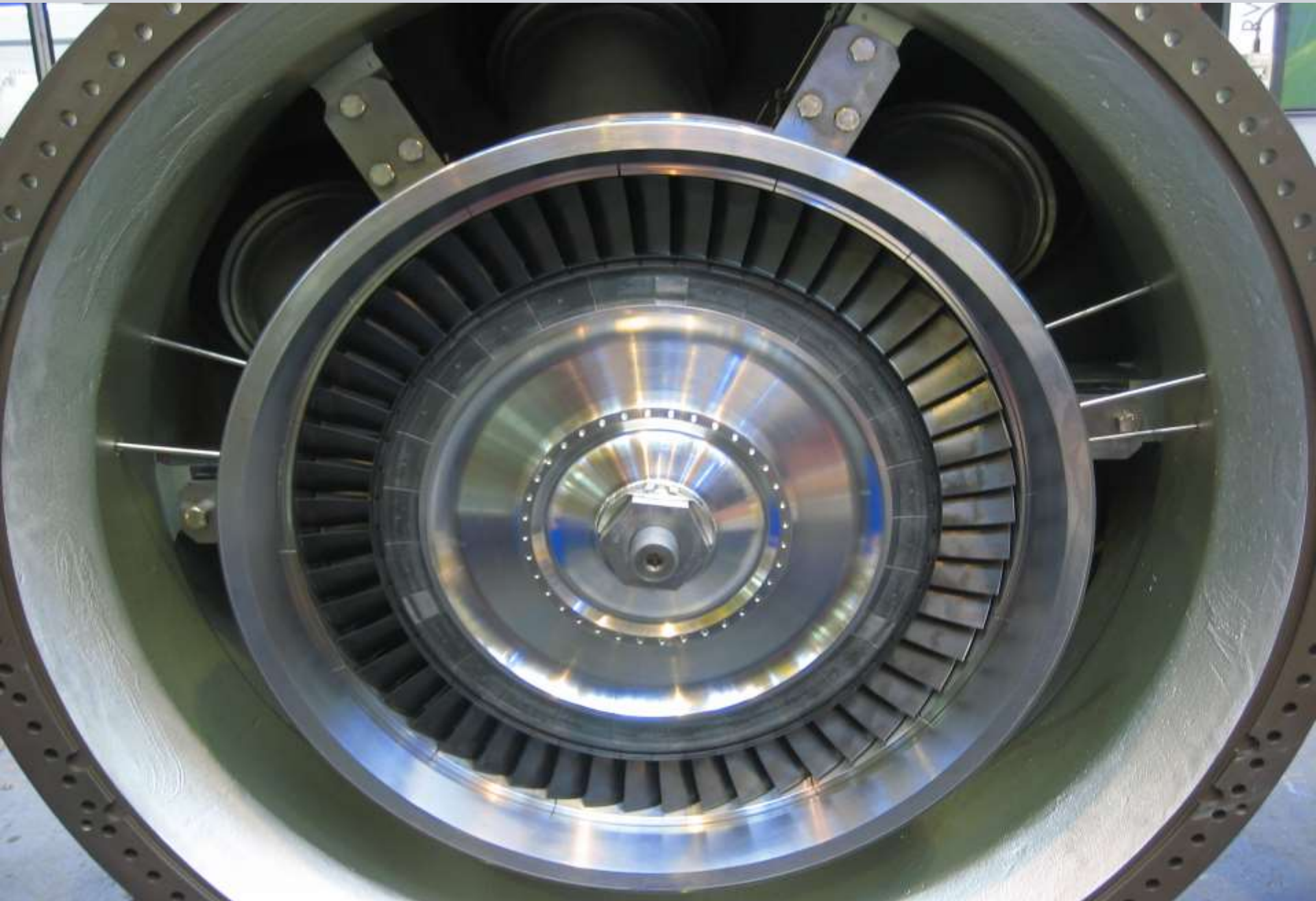
Compressor Turbine CT2 Rotor
