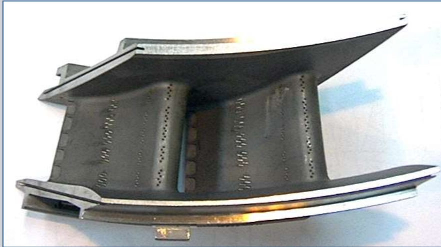
Compressor Turbine Stage 1 Nozzle
