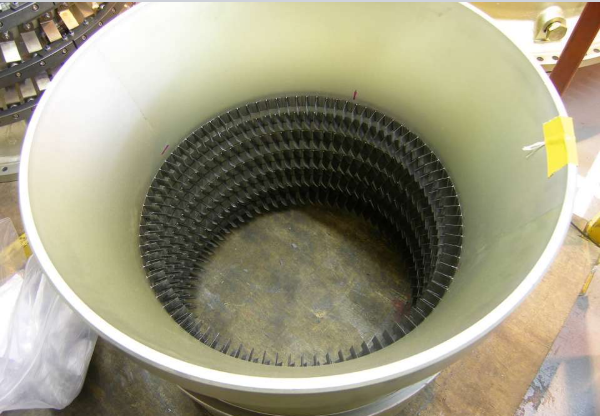
Exit end of SGT400 H P compressor stator.
