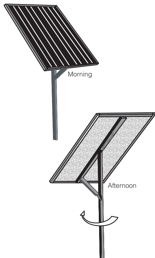
Figure 2.10 Simple manually turned pole-mounted solar tracker
