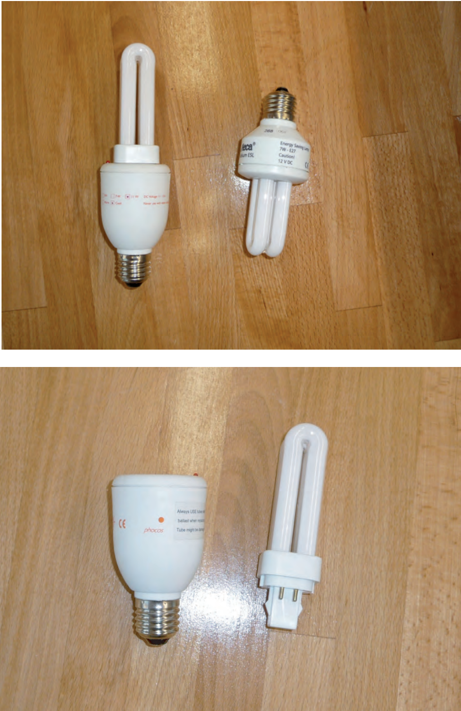
Figure 6.6 'PL-type' fluorescent lamp fittings. Note that in one model (left in top photograph) the bulb can be replaced (the bottom photograph shows how it detaches) – this version is more expensive than the other model (right in top photograph), for which the whole unit needs to be replaced. Care should be taken when selecting the best light fittings for any situation.
