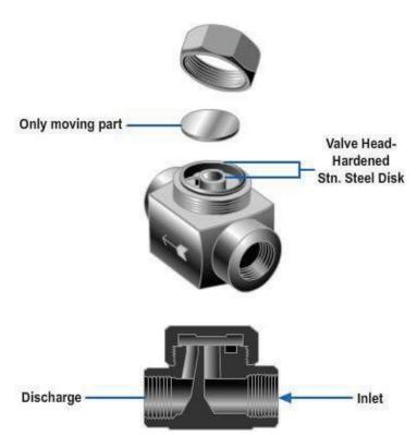
Figure 10-16 — Thermodynamic steam trap.
