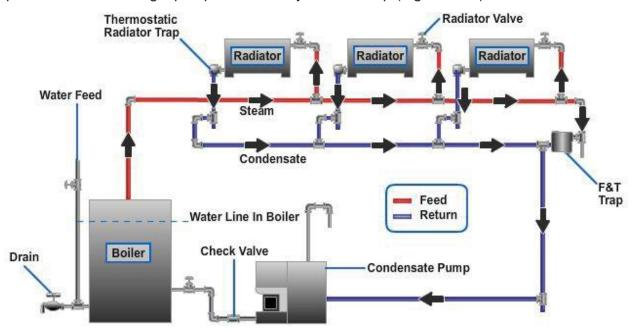
Figure 10-7 — Two-pipe vapor system with a condensate pump.
