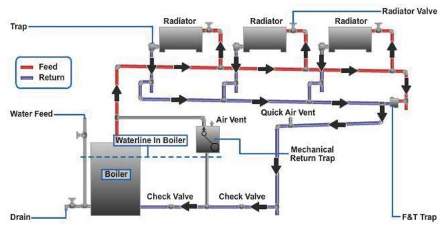
Figure 10-6 — Two-pipe vapor system with a return trap.
