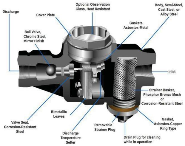
Figure 10-18-Bimetallic-element steam trap.
