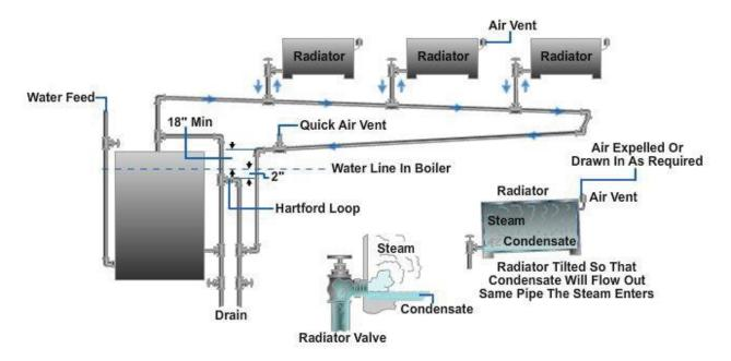
Figure 10-5 — Gravity, one-pipe, air-vent system.
