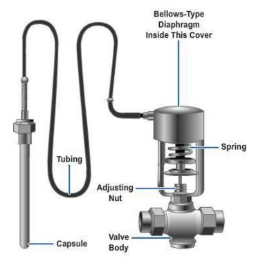
Figure 10-22 - Temperature-regulating valve.
