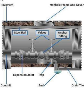
Figure 10-2 — Typical manhole for distribution system.
