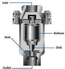
Figure 10-10 — Automatic air vent.
