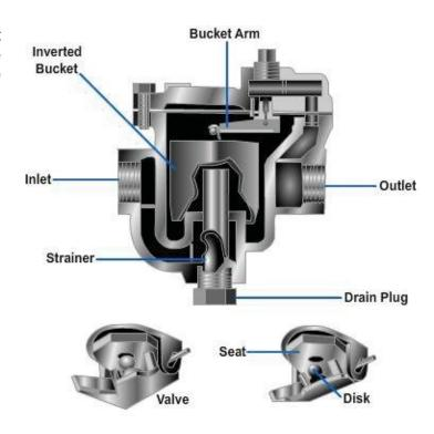
Figure 10-12 — Inverted bucket trap.
