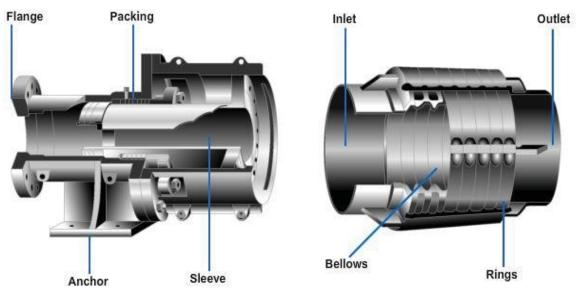
Figure 10-24 — Slip-type expansion joint.
