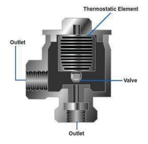
Figure 10-13 — Thermostatic trap.
