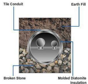
Figure 10-1 — One type of steam distribution conduit.
