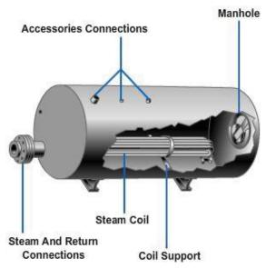
Figure 10-20 – Storage-type water heater.
