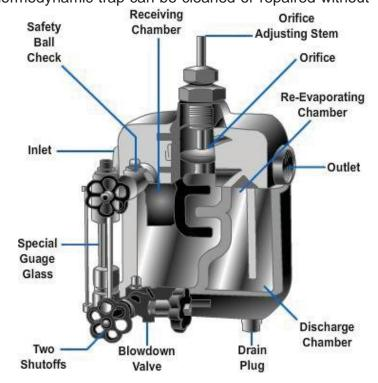
Figure 10-17 — Throttling trap.
