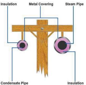
Figure 10-4 — Steam and condensate lines supported by poles.
