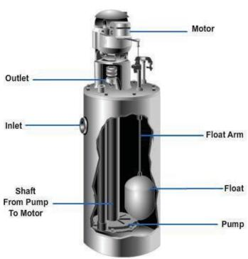
Figure 10-23 — Condensate return pump.
