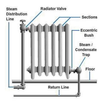
Figure 10-9 — Cast-iron radiator.
