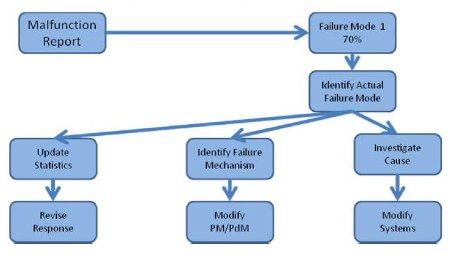
The updated statistics will identify the Failure Mode that is most likely and should be the first target of the troubleshooter. Addition of new Failure Mechanisms or current Failure Mechanisms appearing in new locations suggests the addition of new Predictive or Preventive Maintenance. Once the cause is understood, it may be possible to alter the organization, procedures or processes to prevent reoccurrence.
