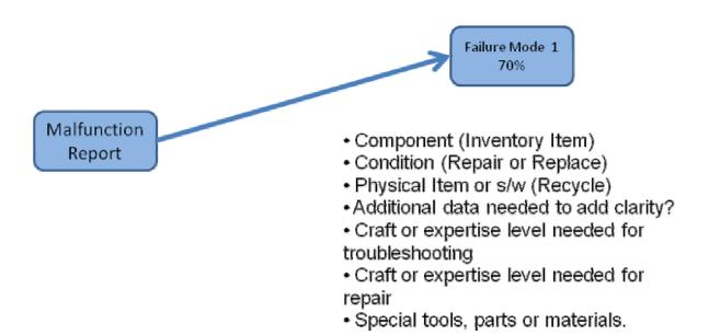
The Failure Mapping database should store information associated with each Failure Mode to facilitate rapid recovery.
