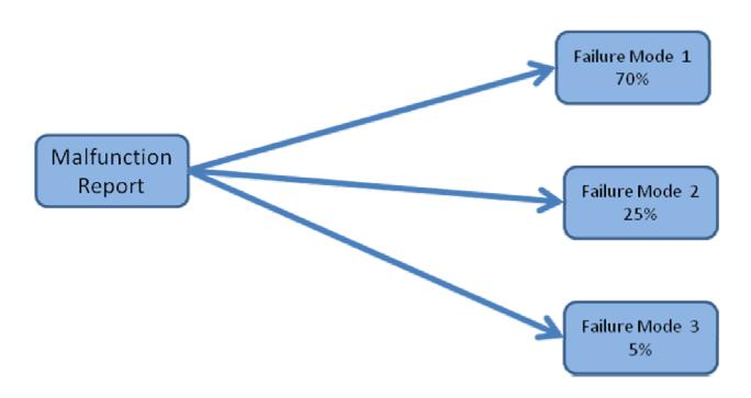
The Failure Mapping database should identify the link between each Malfunction Report and all the Failure Modes that could cause it along with the historical frequency of their occurrence.
