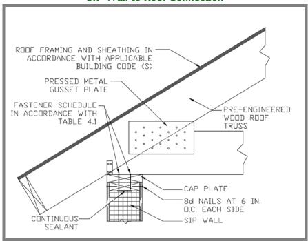
Figure 4.3 SIP Wall to Roof Connection
