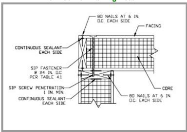
Figure 6.3 SIP Corner Framing Detail
