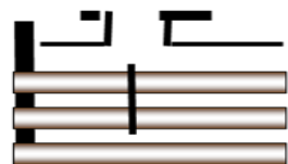
Inlet support baffles
