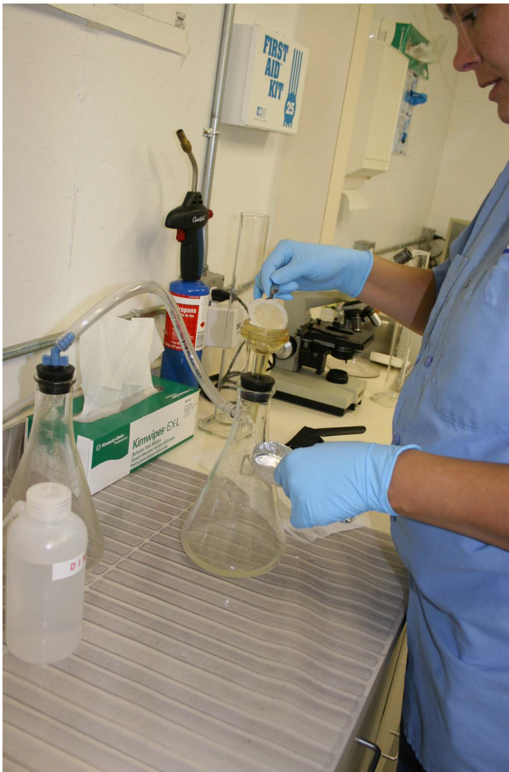
Lab tech removing filter for TSS analysis.
