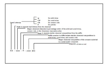
Figure 3-1. Thermal spray feedstock designation nomenclature
