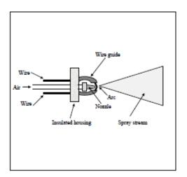
Figure 2-7. Typical two-wire arc spray gun
