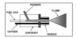
Figure 2-5. Powder gun cross section
