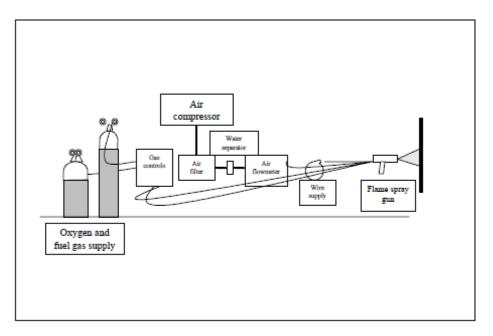
Figure 2-2. Typical flame spray system
