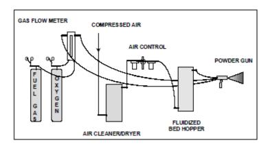
Figure 2-4. Typical combustion powder gun installation
