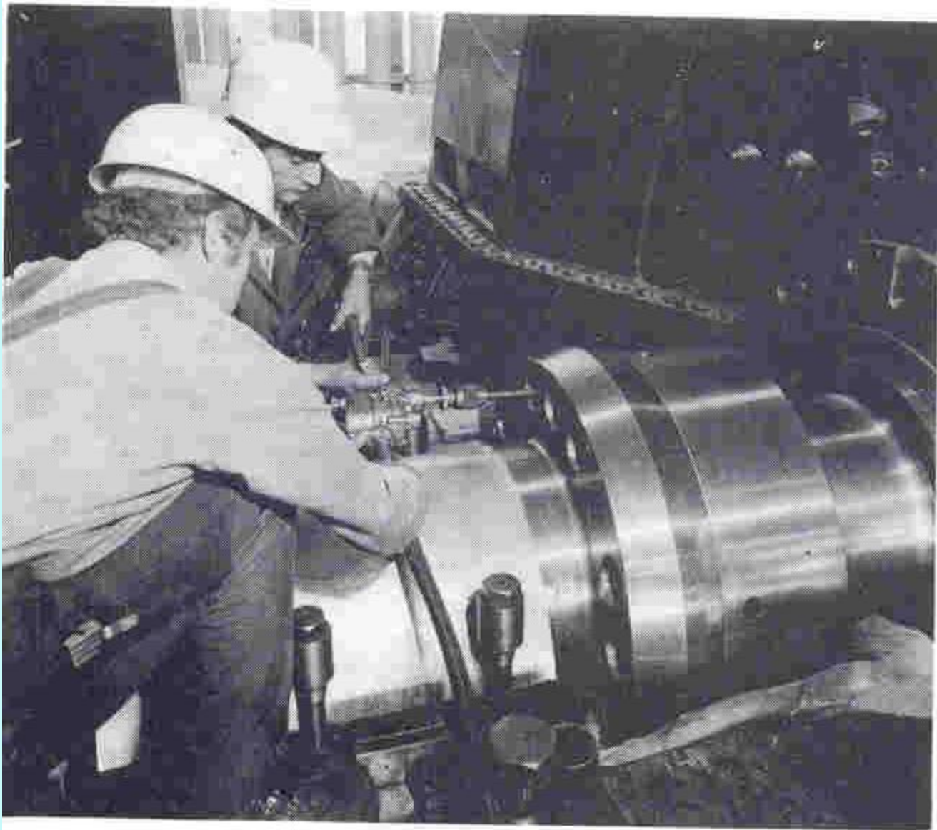
fig. 4 Honing the Holes for the Coupling Bolts
