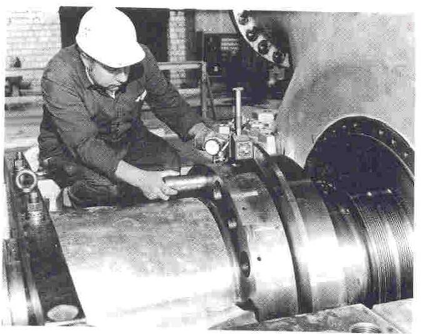
Fig. 3 Checking and Drawing Together Coupling Heads
