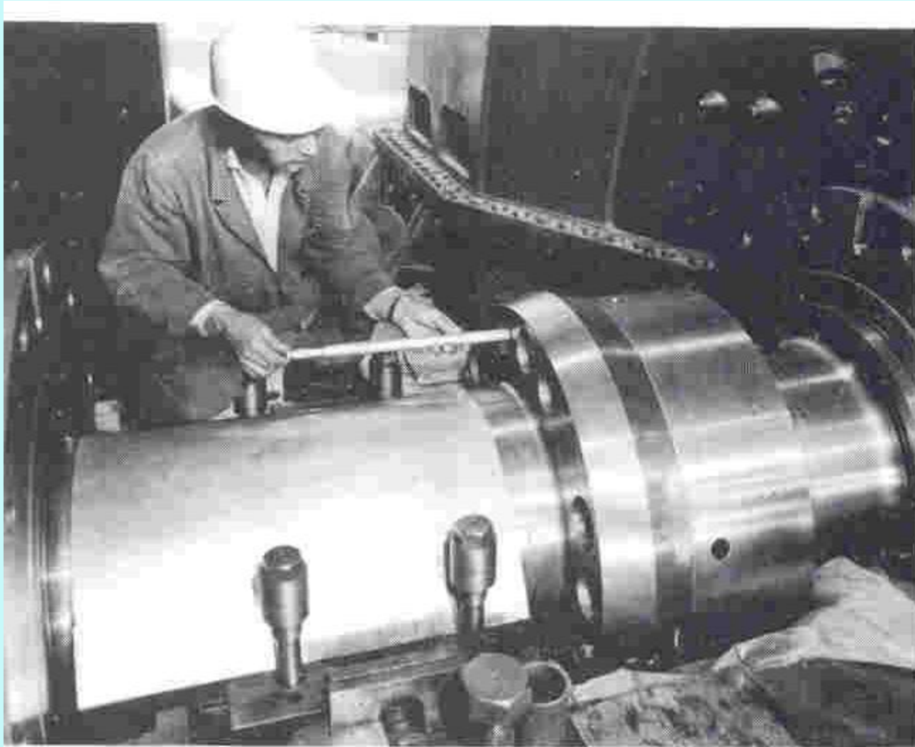
Fig. 5 Measuring the Coupling Bolt Holes Using a Three-Point Gauge
