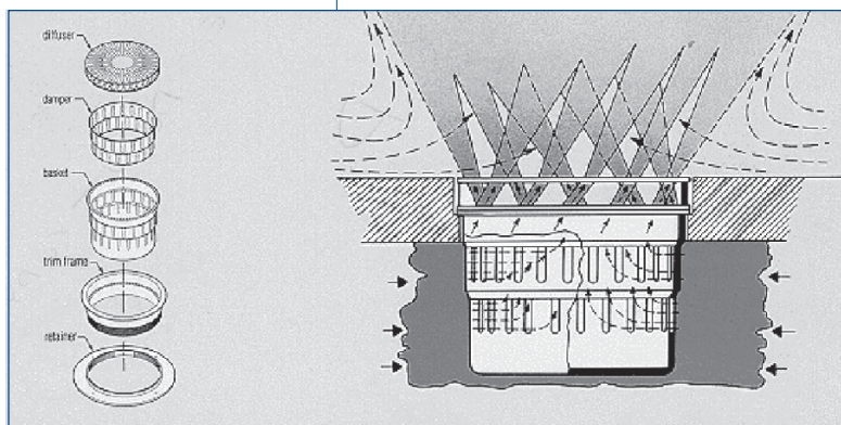
Illustration of typical swirl diffuser used in UFAD systems.
