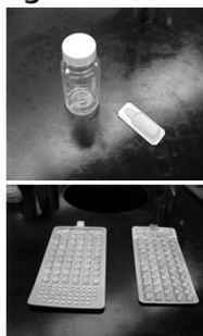
Colilert media® and sample bottle (top) and results after incubation in QuantiTrays® (bottom).
