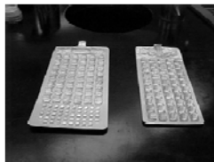
Left: The 96 well QuantiTray 2000 will count up to 2419 cfu without dilution. Right: The 51 well QuantiTray will count up to 200 cfu without dilution.
