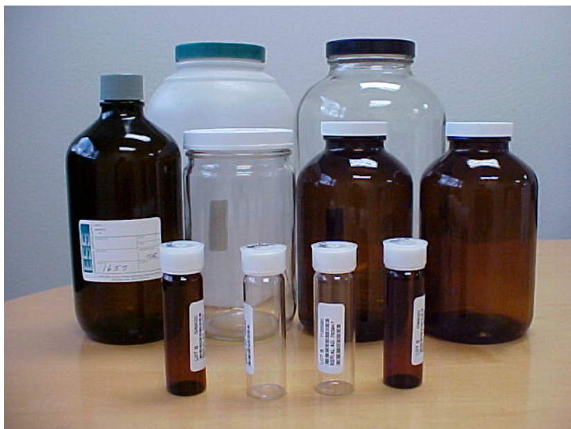
Common Wastewater Sample Collection Bottles Above, 625/608, 1657, TTO/Organics, TPH/Oil/Grease Smaller bottles-TOCs, VOCs, 601/602 and 502.2.
