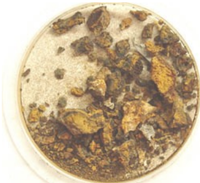
Large Rust Particles
