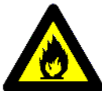
Flammable material or high temperature
