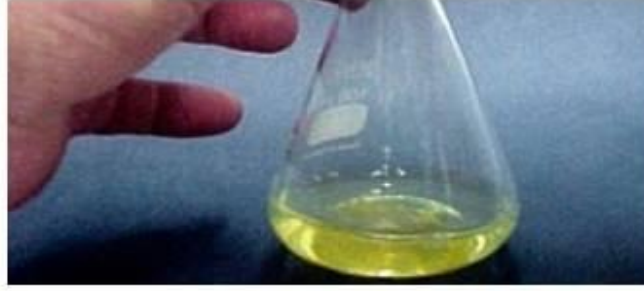
Figure 1 Before the addition of any silver nitrate the chromate indicator gives the clear solution a lemon-yellow colour.
