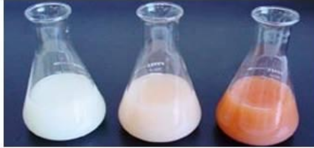
Figure 2 Left flask: before the titration endpoint, addition of \text{Ag}^+ ions leads to formation of silver chloride precipitate, making the solution cloudy. The chromate indicator gives a faint lemon-yellow colour. Centre flask: at the endpoint, all the \text{Cl}^- ions have precipitated. The slightest excess of \text{Ag}^+ precipitates with the chromate indicator giving a
