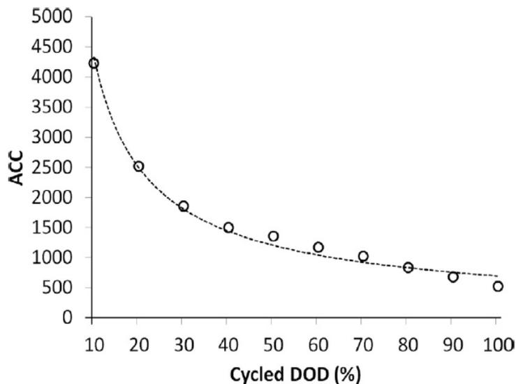
Figure 4: Illustration of  $ACC(DOD)$  function for a lithium-ion battery
