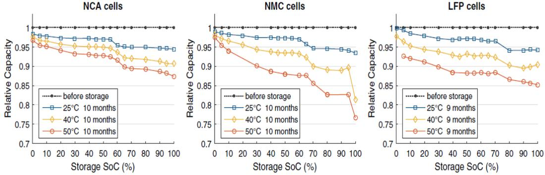
Figure 5: Results of accelerated calendar aging tests at various SOCs and temperatures
