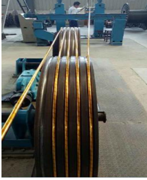
Fig. 3. Photo of 100 m HTS composite cable in insulation coating process.
