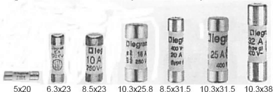
Figure 48: Cylindrical fuses – IEC Standards – Domestic type – sizes in mm
