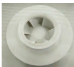
Figure 20. 3D wax pattern.
