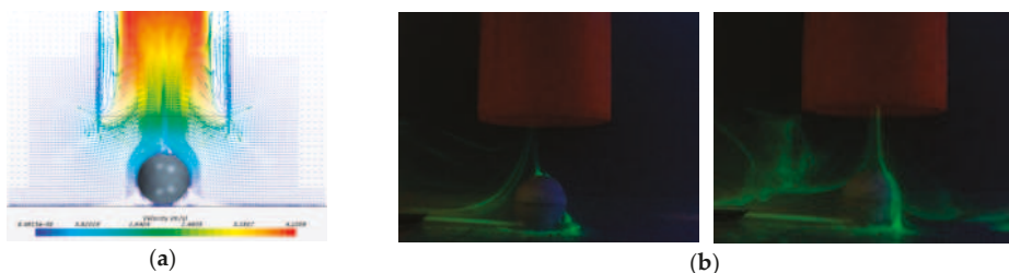
Figure 17. (a) Velocity vector distribution from numerical solution ( h = 0.07 m, v = 2 m/s, Re = 61162 ) [16]; (b) Flow visualization results ( h = 0.07 m, v = 2 m/s, Re = 61162 ).
