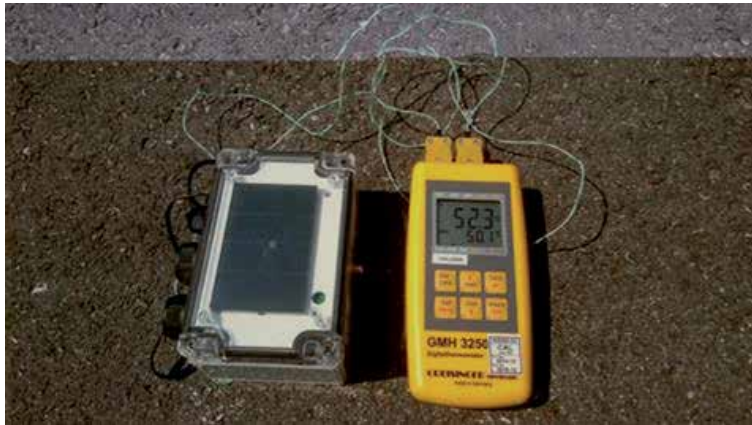
Figure 6. Measuring temperature inside the EnOcean low power, energy harvesting sensor module housing. The two channels of the thermometer (yellow device) are measuring the temperature of the solar cell (52.3°C) and supercapacitor (50.1°C), respectively. The outside temperature was 30°C.
