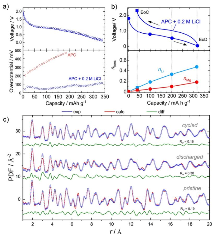
**Figure 3.** **a)** Galvanostatic-intermittent-titration-technique performed during the first discharge (bottom) and evolution of the overpotential during the first discharge with (APC +0.2M of LiCl) and without (APC) lithium. **b)** Chemical analyses (ICP-AES) of Li, Mg contents during the first cycle. The electrolyte was APC with 0.2M of LiCl. **c)** Refinements of the PDF data of pristine, discharged and cycled electrodes.
