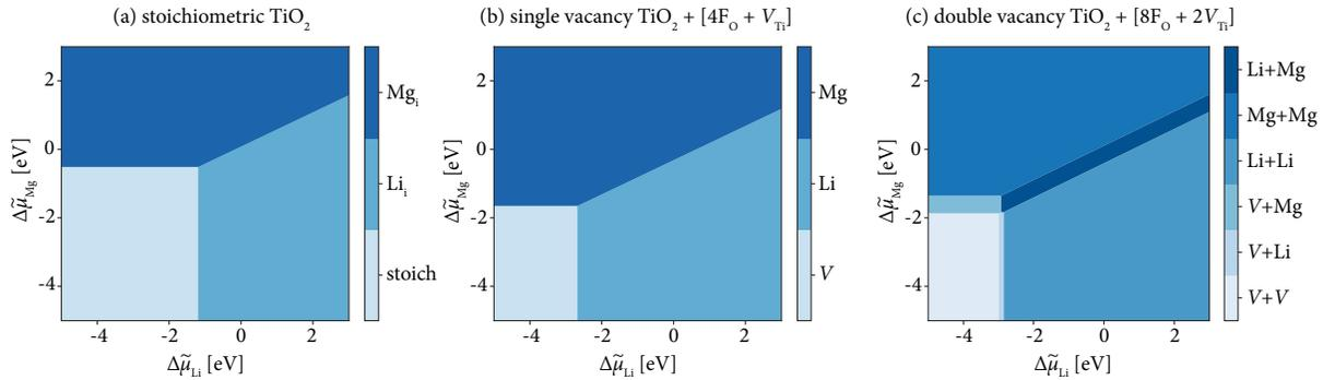
**Figure 6.** The lowest energy intercalation products at a paired  $V_{\text{Ti}}+V_{\text{Ti}}$  site, as a function of magnesium and lithium electrochemical potentials relative to the elemental metals;  $\Delta\mu_{\text{Mg}}$  and  $\Delta\mu_{\text{Li}}$ ), calculated from DFT data. *Source:* source data, figure files, and plotting scripts are available under the CC-BY-4.0 license as part of reference [39].
