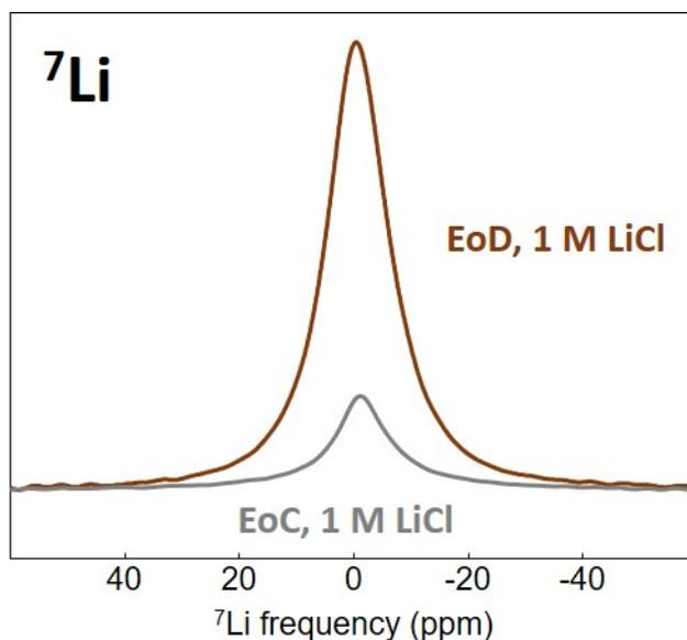
**Figure 5.** Expansions of the central lines of the non-normalized  ${}^7\text{Li}$  MAS (44 kHz) NMR spectra of the electrochemically discharged (EoD) and charged (EoC) electrodes using hybrid electrolyte 0.2 M APC + 1 M LiCl.
