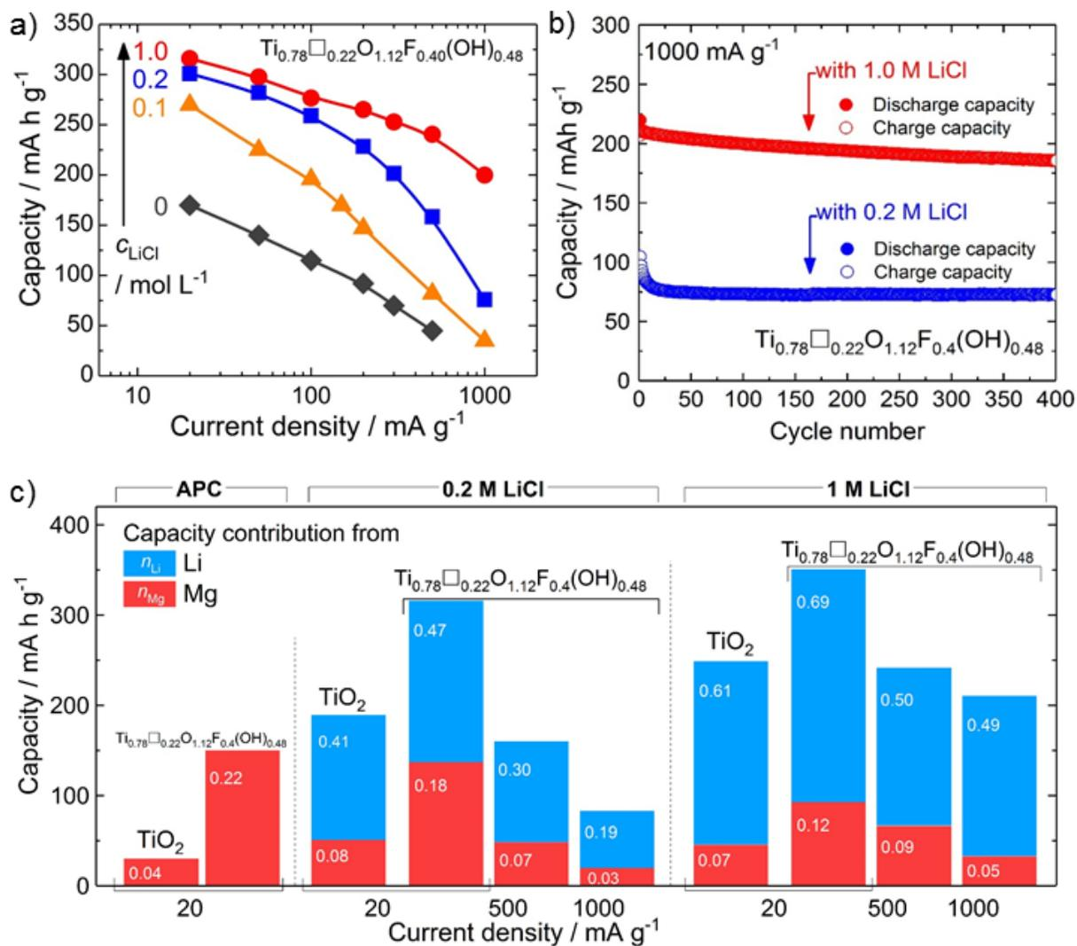
**Figure 2.** a) Rate capability plots of  $\text{Mg}/\text{Ti}_{0.78}\square_{0.22}\text{O}_{1.12}\text{F}_{0.40}(\text{OH})_{0.48}$  cells cycled with different lithium concentrations. b) Long term cycling of  $\text{Mg}/\text{Ti}_{0.78}\square_{0.22}\text{O}_{1.12}\text{F}_{0.40}(\text{OH})_{0.48}$  cells under  $1000 \text{ mA g}^{-1}$  with
