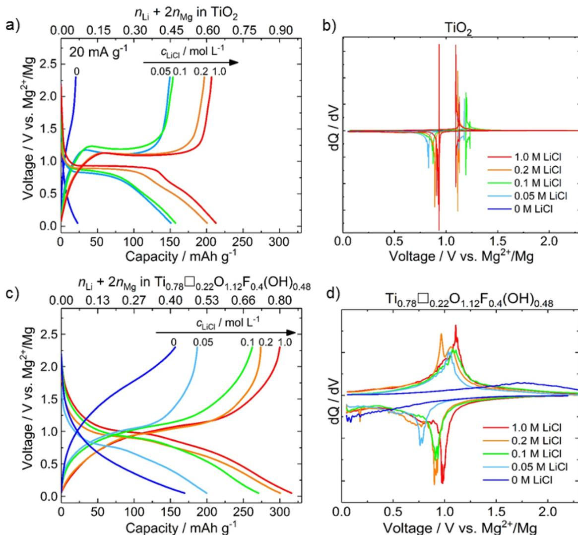
**Figure 1.** Discharge–charge curves and corresponding derivative curves for Mg/TiO<sub>2</sub> (**a,b**) and Mg/Ti<sub>0.78</sub>O<sub>1.12</sub>F<sub>0.4</sub>(OH)<sub>0.48</sub> (**c,d**) cells cycled at 20 mA g<sup>-1</sup> using 0.2 M APC with various LiCl concentrations. The discharge-charge curves were obtained after two cycles of activation.
