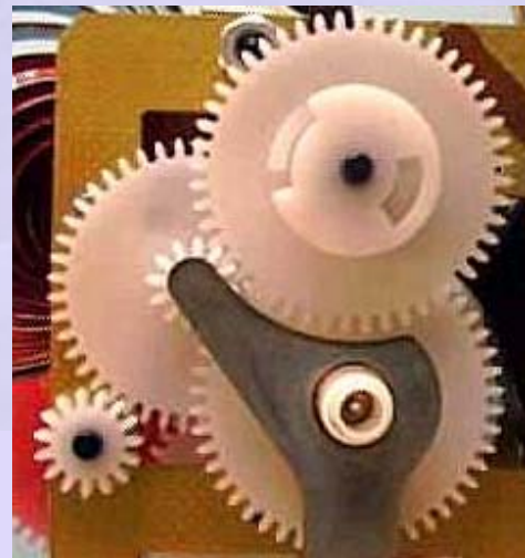
Fig. 1.30 Application of cycloidal tooth gear in a clock mechanism
