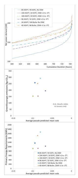
Fig. 9: Performance of SOFC-mCHP systems
