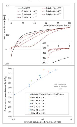
Fig. 8: Performance of ICE-mCHP units
