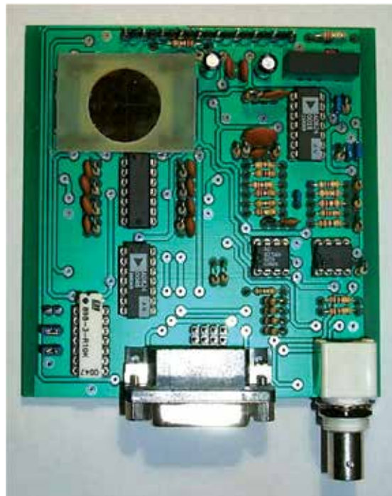
Fig. 22. Electronic board of the module PosIRix. In the bottom side, the DB5 type connector for the instrument V-Bus connection is sided in a central position; on the left side is shown the BNC connector for laser pulse monitoring by an oscilloscope. On the top left a 28mm x 28 mm PVDF four quadrant sensor with a circular ZnSe window for spectral filtering the CO 2 wavelength.
