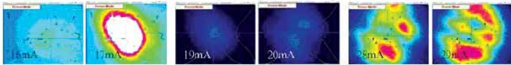
Fig. 18. The far-field pattern of 850 nm VCSEL as function of injected currents, oxidized times of 70 min
