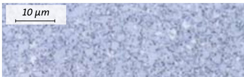
Fig. 3.5: Micrograph showing surface of tungsten carbide
