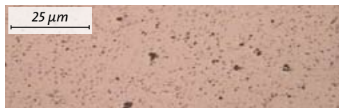
Fig. 3.3: Micrograph showing surface of alumina
