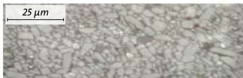
Fig. 3.4: Micrograph showing etched surface of alumina
