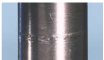
Fig. 5.18: Corrosion on shaft below dynamic O-ring caused by axial movement of the shaft
