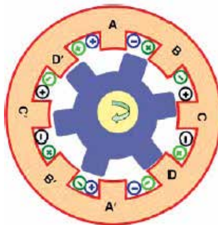
Figure 5. A switched-reluctance motor with 8 stator poles and 6 rotor poles
