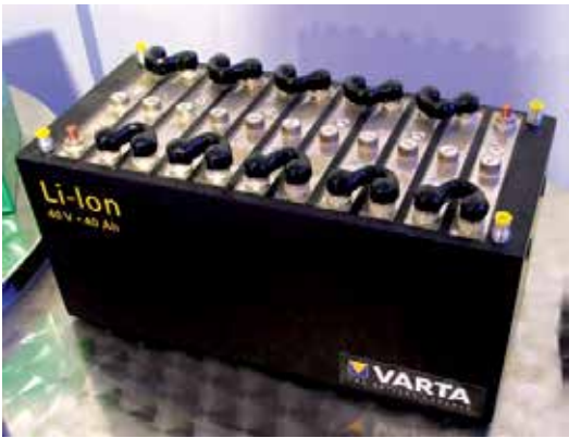
Figure 22. A typical Li-ion battery pack utilized in the EVs [21].
