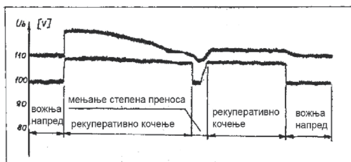
Figure 8. Change the battery voltage during DC recuperative braking in [15, 16].
