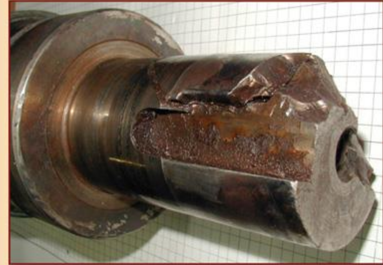
Photo 7. The terrible (loose) coupling fit on this motor shaft allowed the hub to repeatedly drive the key against the side of the keyway until a fatigue crack developed.
