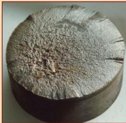
Photo 5. The shaft on this 200 hp, 1180 RPM motor failed in less than a day as a result of badly worn sheaves on the belt drive.
