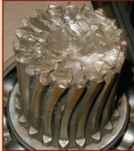
Photo 1. This shaft has been grossly overloaded by a torsional stress.
