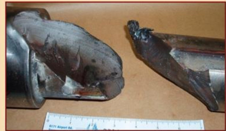
Photo 8. The torsional fatigue failure of this fan shaft occurred shortly after the installation of a variable speed drive.
