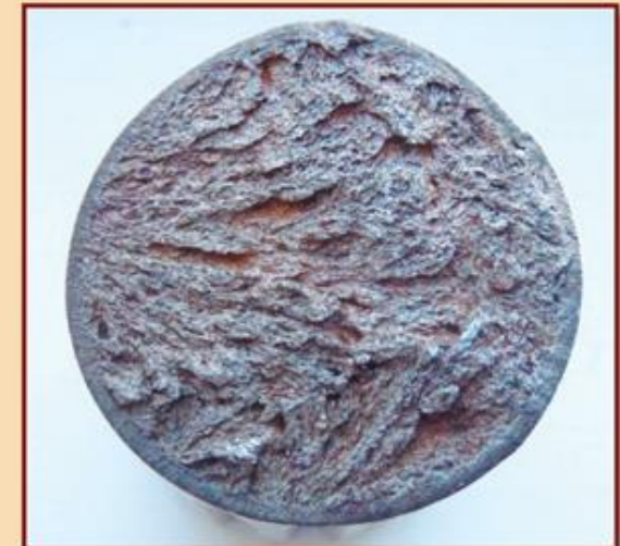
Photo 4. This case-hardened splined section of a hydraulic pump shaft shows evidence of a brittle fracture caused by a single bending force.
