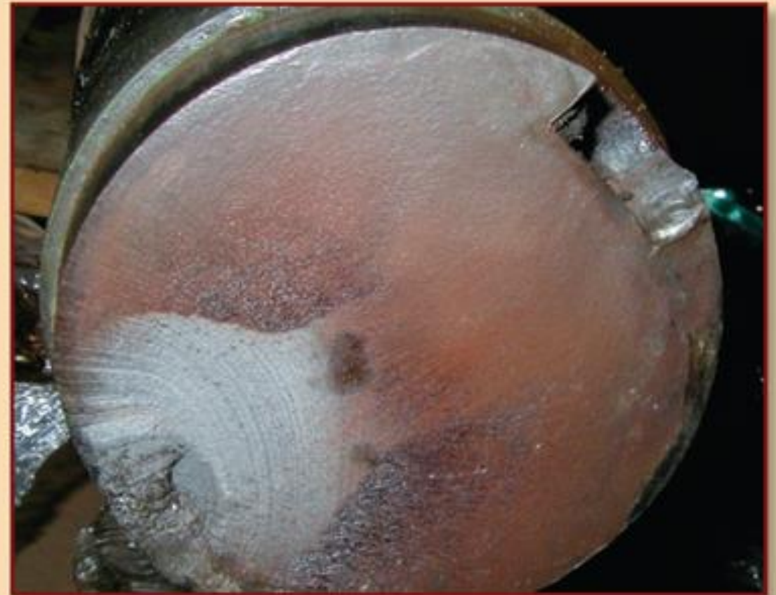
Photo 6. This slow-growing failure on a steel-mill elevator drive was initiated by fretting corrosion that substantially reduced the fatigue strength on the shaft.
