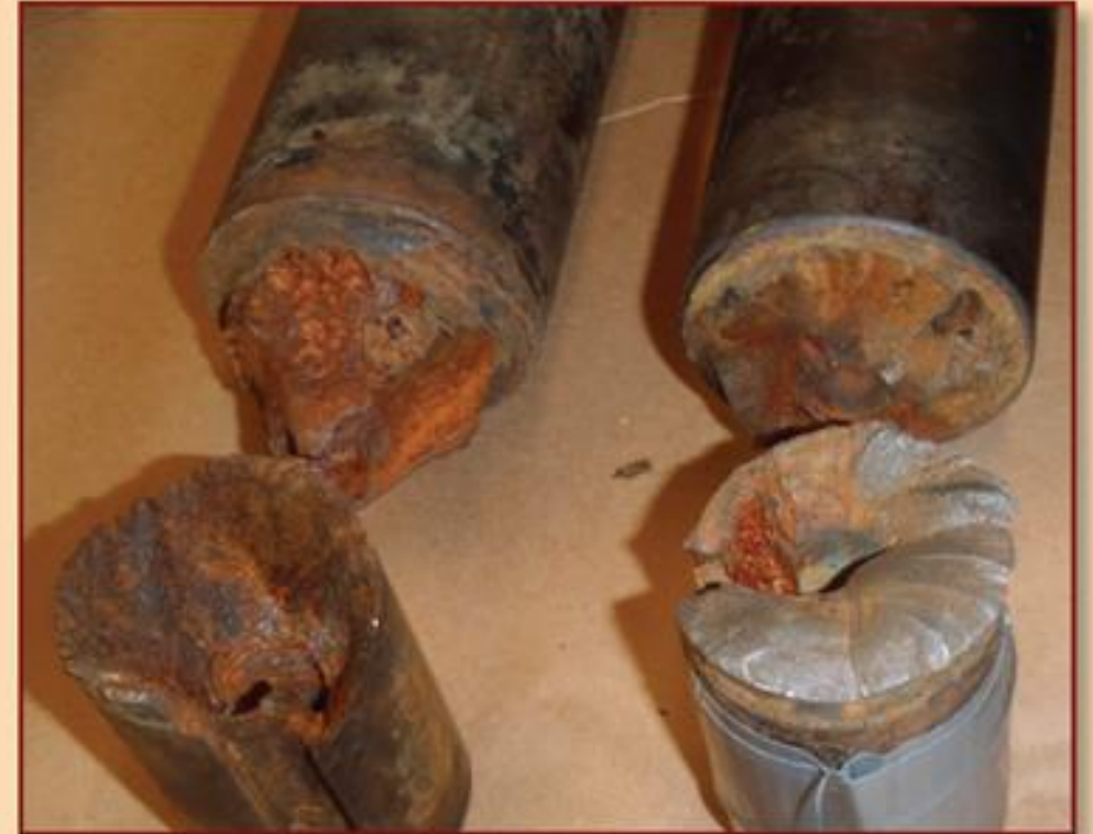
Photo 9. These pump shafts failed due to torsional fatigue aggravated by the reduction in strength caused by corrosion, not because of rotating bending.
