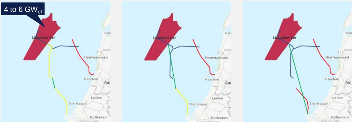
Case study for connecting IJmuiden Ver to the Maasvlakte 2 . The left picture is for a 400 MW el offshore electrolyser, the middle for 1 to 2 GW el (required pipeline diameter: 16", resp. 36"), the right picture is for > 2 GW el . Yellow lines are reused natural gas pipelines, green lines are newly built hydrogen pipelines. Source: DNV
