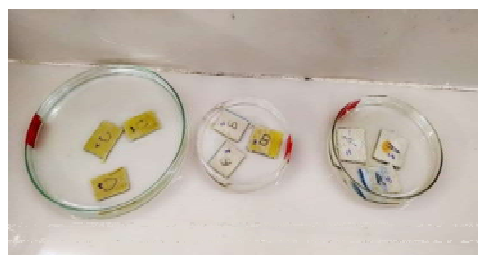
Figure 4. Specimens for the water absorption test using the ASTM D-570 standard.
