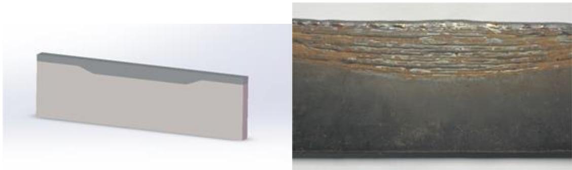
Figure 32 Height varying deposition experiment (Xu et al., 2019) a. schematic diagram for pre-define uneven substrate with height-varying deposition b. deposition result.
