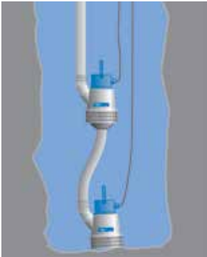
The head generated can be increased by connecting two or more Type BS - Pumps in series
